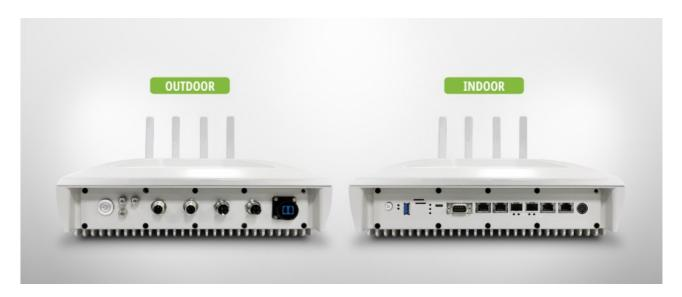
The CASwell MEC-6300 will be offered in two versions – one for using indoors and one for outdoor
